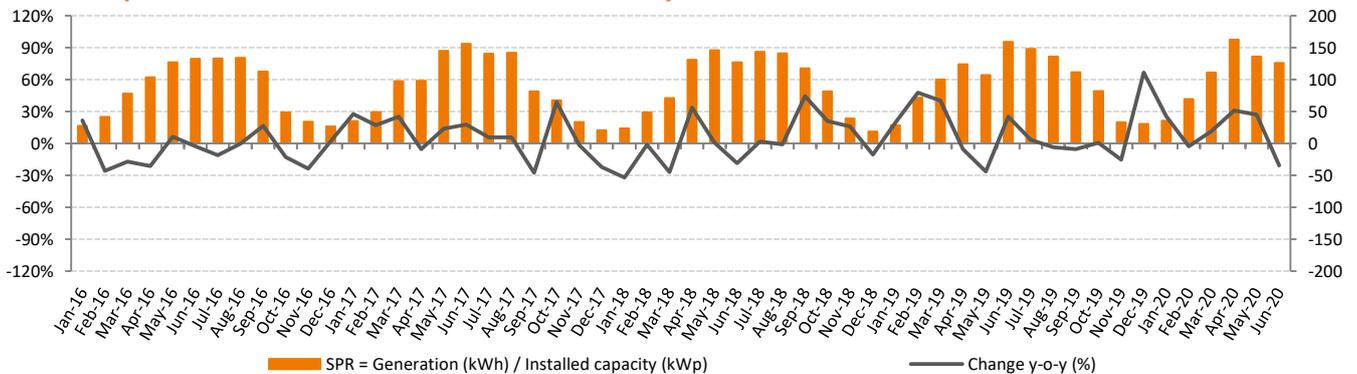
Specific Performance Ratio is a measure of efficiency which shows the amount of kWh generated per 1 kWp of installed capacity and enables the simple comparison of year-on-year results and seasonal fluctuations during the year.
